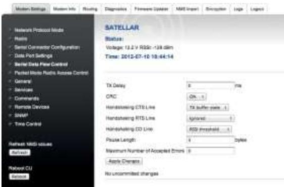
Figure 7.9 Serial Data Flow Control view; WWW interface
